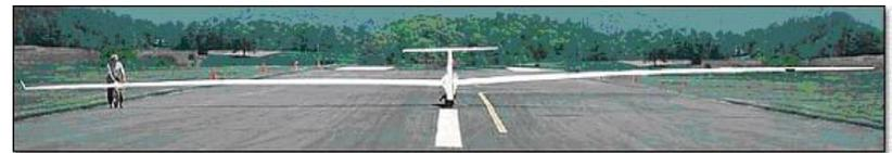
Modern gliders (like the ASW22 pictured above) have glide ratios of around 60 to 1 in still air; therefore if the glider is 1000m (3280 feet) above ground it can glide for 60km before meeting the ground.
