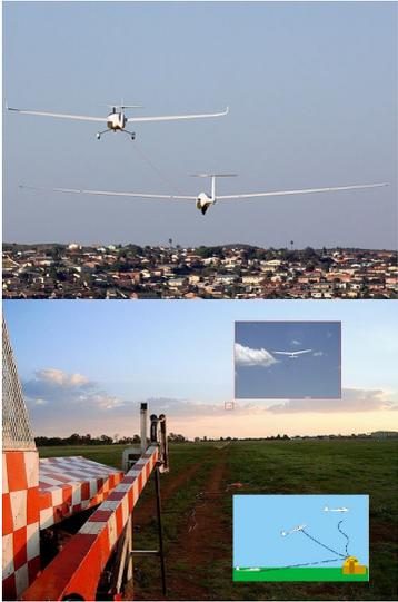
To begin a flight a glider must achieve its initial height (potential energy) and launching a glider is done with the use of some outside energy. There are two predominant means of launching a glider: Aero tow and Winch launch. At EPGC we mainly winch launch, but aero tows are available from time to time.
