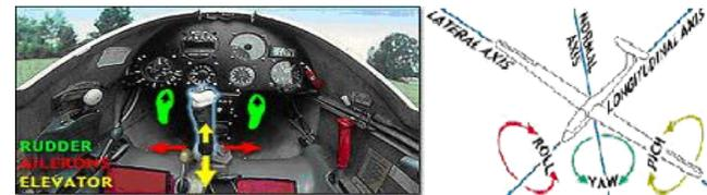
A glider, as with most aircraft, has three primary control surfaces: **RUDDER**, **AILERONS** and **ELEVATOR**. The pilot thus has the ability to control all 3 axes of the aircraft.
